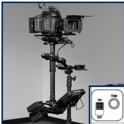
The pause switch is there to keep the Volt powered on and tracking the encoder and motor positions.
