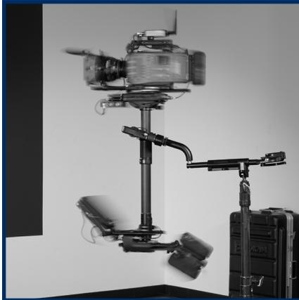
Then, change the balance to be completely neutral top-to-bottom. It should hold any post angle and not rotate.
