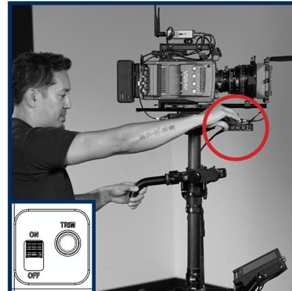
IF the control box is mounted for regular operators (knobs on the RIGHT) align the gimbal handle with the REAR of the post and simultaneously power on the Volt. Wait 2.5sec while the system registers the pan encoder position.
