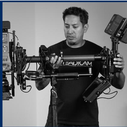
Make sure the sled does not pan when holding a tilt. If so, a tiny adjustment to your side-side balance should correct this.
