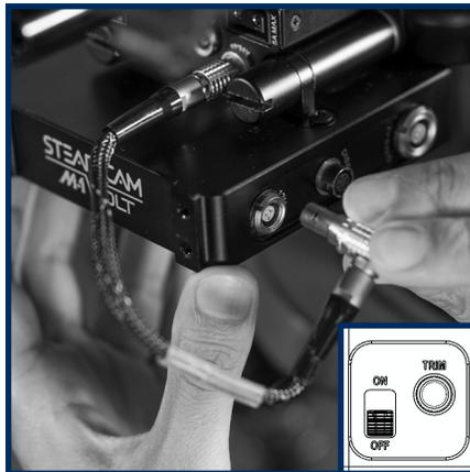
Plug in the Volt gimbal cable and wrap a couple of loops around the post as needed to control any slack.
