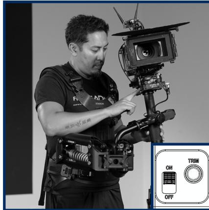
To reset the roll horizon to default, LONG-press the trim button on the control box for 6 seconds until both LEDs on the control box turn off and pulse back on.
