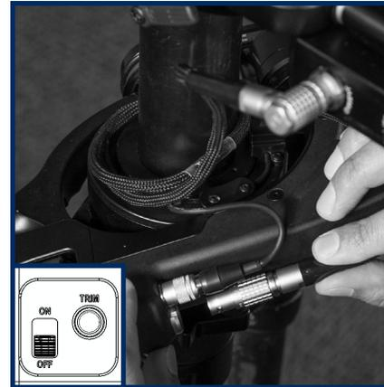
**Your Volt equipped sled should now be ready for action! Flip back to page 7, and get ready to balance before powering on.**
