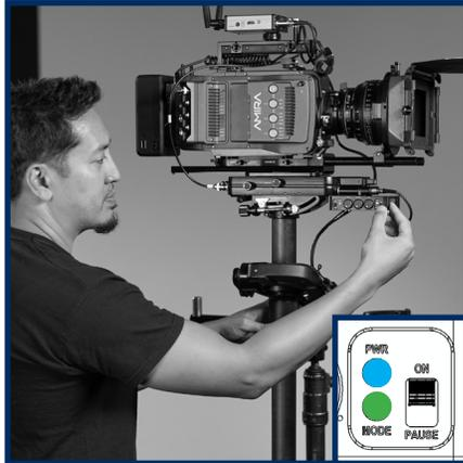
The Volt only needs to have the post encoder aligned when powering on.
