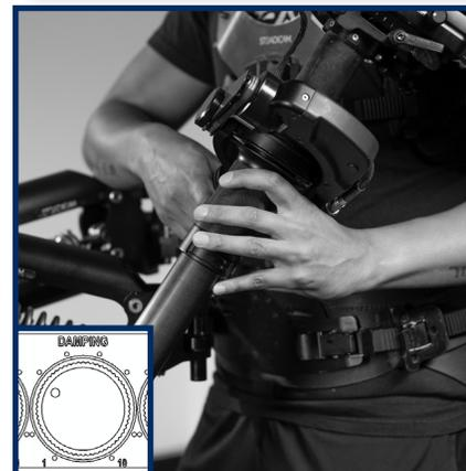
Damping works like friction to keep the sled from oscillating.
