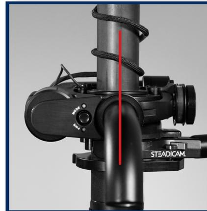
**REMEMBER:** If your box is mounted with the knobs to the RIGHT (regular), you'll align the gimbal handle to the REAR when powering on later.
