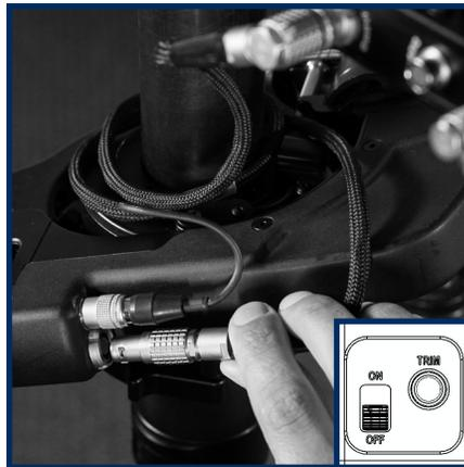
Make sure the pause switch is DOWN, indicating the Volt motors will not run.
