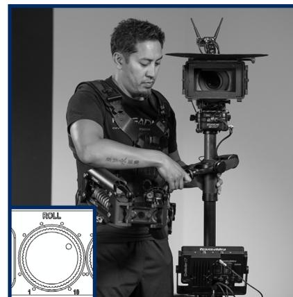
The ROLL dial controls the strength of the motors in the roll axis. This equates to how strongly the rig seeks a level horizon side-to-side.
