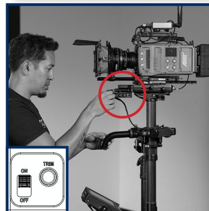
IF the control box is mounted for goofy operators (knobs on the LEFT) align the gimbal handle with the FRONT of the post and simultaneously power on the Volt. Wait 2.5sec while the system registers the pan encoder position.
